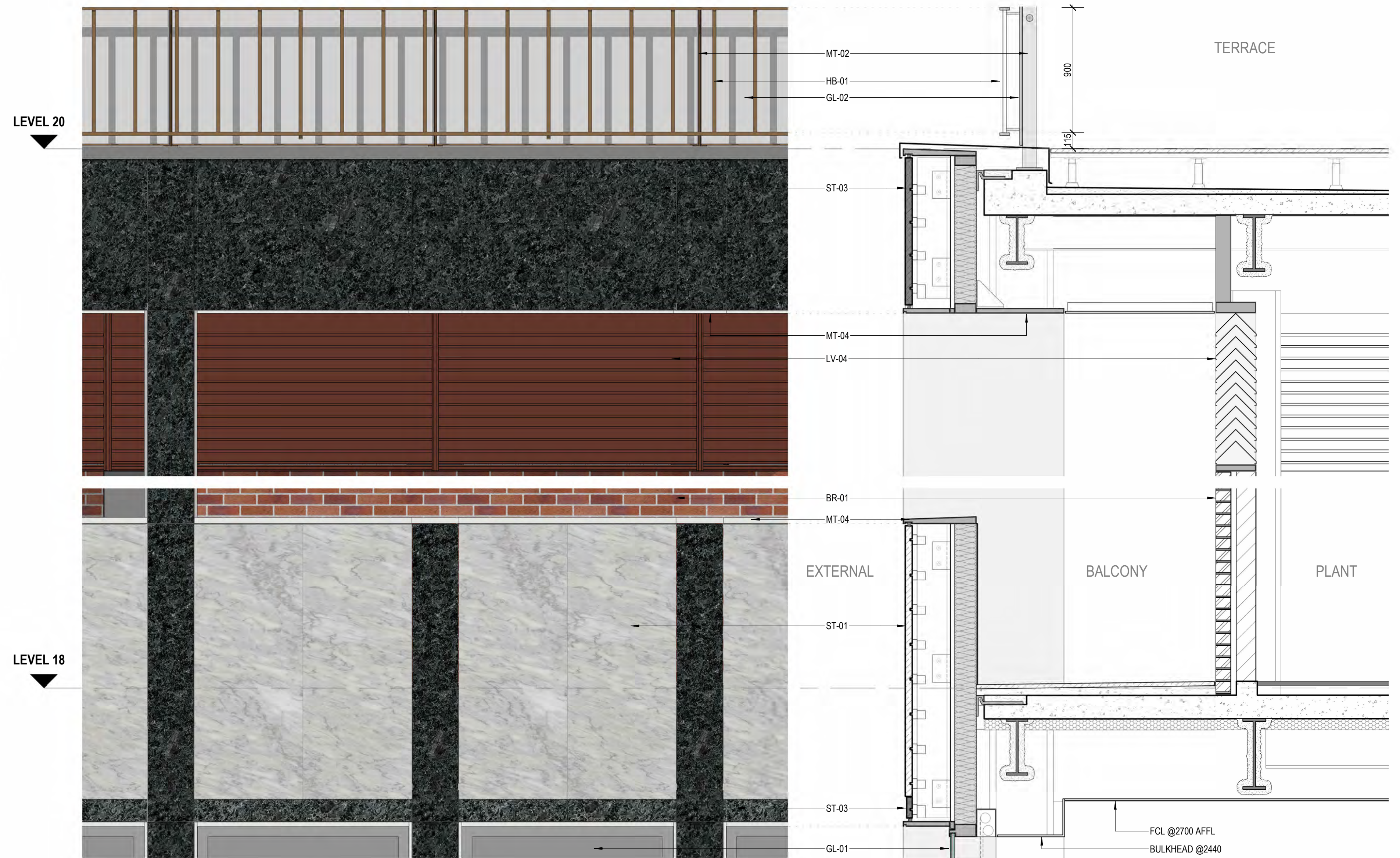
2 Level 18 Plant Room Detail Elevation SCALE: 1 : 20
